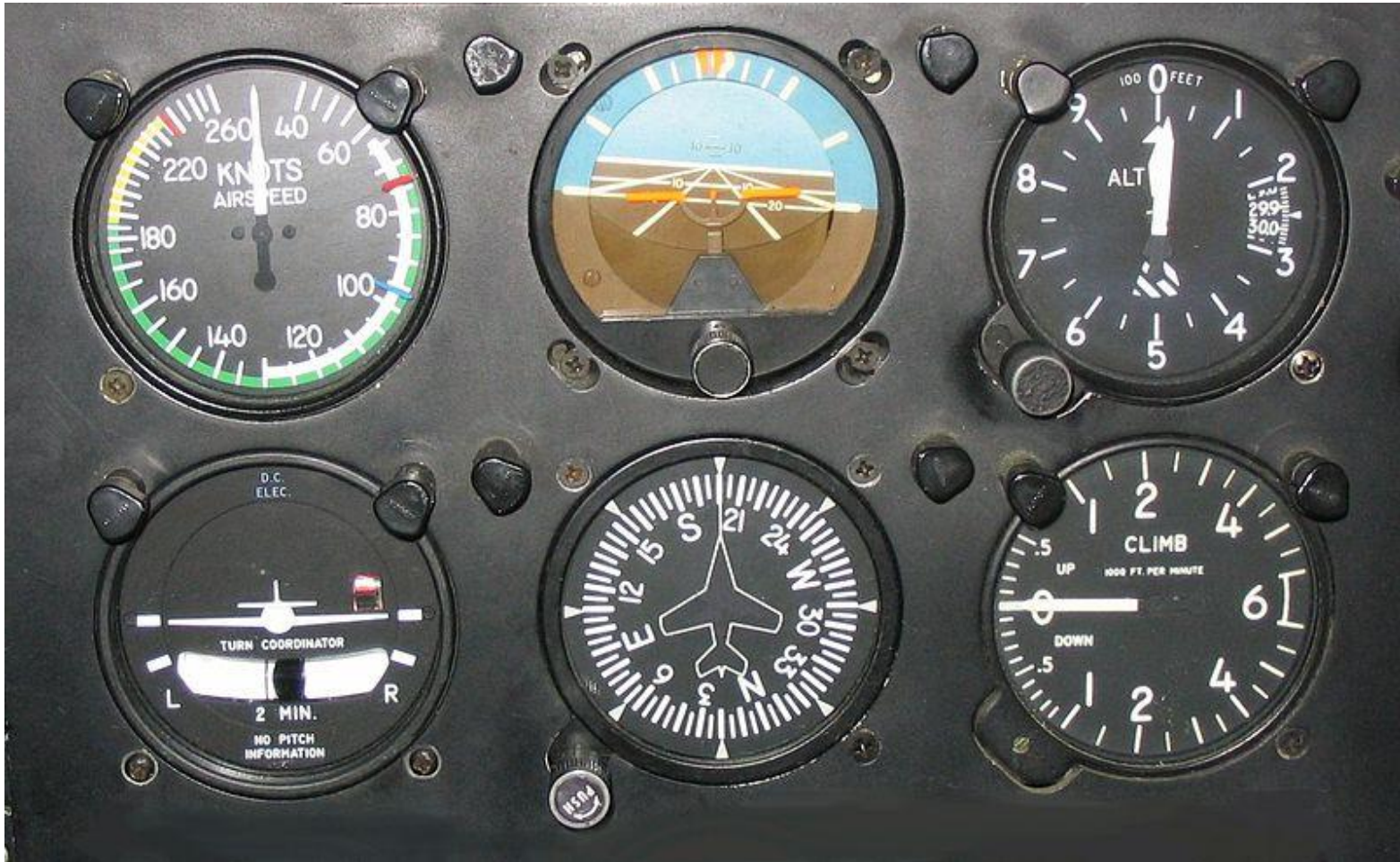
Airspeed Indicator, Attitude Indicator, Altimeter, Turn and Bank Indicator, Heading Indicator, Vertical Speed Indicator
